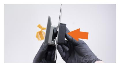
Now **place the lid on top of the liquid container** so the print is **submerged** in isopropyl alcohol. This is the recommended procedure, because both the platform and the object are washed. If the object is too large for the tank, remove it from the platform and wash it twice - first in "normal" orientation, then rotate it upside down and wash it again.
