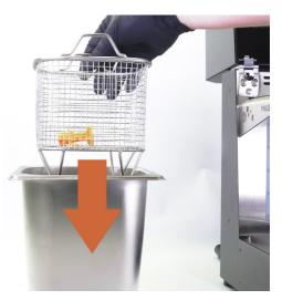
If you printed a **large object that doesn't fit the container**, wash it in two stages: first, submerge it in IPA as usual and run the washing process. Then, take the object out, rotate it upside down and put it in IPA again to wash the part that wasn't submerged in the first run.
