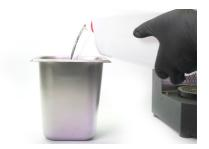
Prepare the **stainless steel tank** and the **magnetic propeller**. Place the magnetic propeller into the tank so it lays flat on the bottom. Blades must point upwards.
