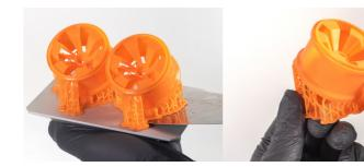
Use a metal spatula to remove the printed object from the printing platform. You can also consider removing the supports at this point.
