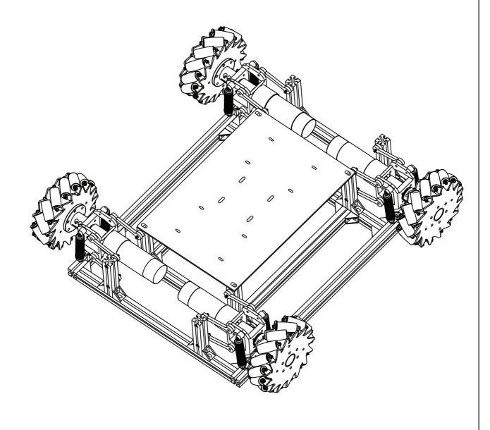
13. Finally, we will mount the Top Plates to the chassis frame with the help of M4 Button Head Allen bolt & Sliding Nut.
