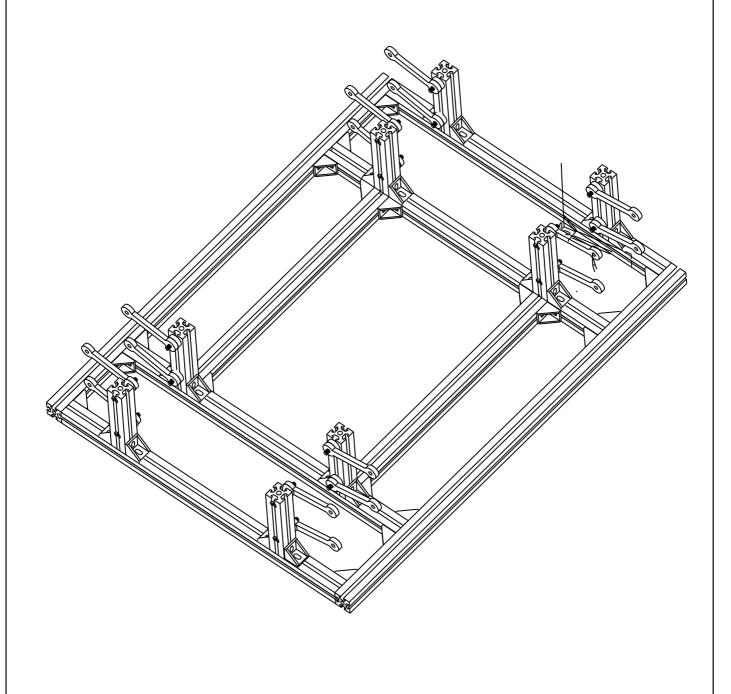
6. Mount 8 pieces of Corner bracket along the length of 550mm extrusion as shown below. Make sure it is mounted correctly as per dimension shown in image. (Note – All dimensions are in mm)
