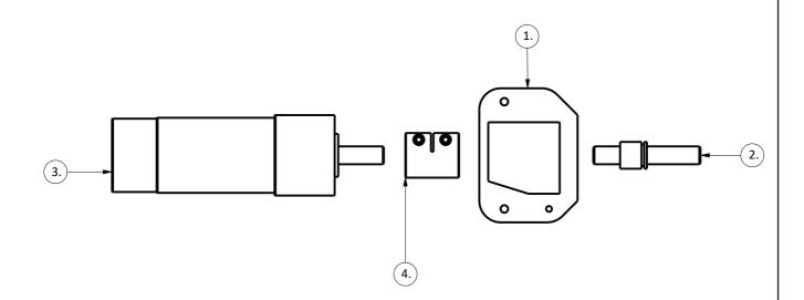
9. Now, we will fix Drive Assembly set up to the frame. This step is quiet hard compare to other steps. Fix the Drive Assembly carefully. Use 5mm spacers & M4 Allen Bolt with Nyloc Nut for linkages & 10 mm spacers & M3X25 Allen bolt with Nyloc Nut for Shock Absorber. Tight the all Linkages by making sure that Shock Absorber Spring compress & expand freely.
