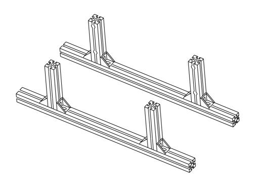
3. Next, take 2 pieces of 550mm length 20X20 extrusion as fix them as shown in fig. Make sure orientation of the extrusion while fixing the extrusion. Make sure it looks symmetric.
