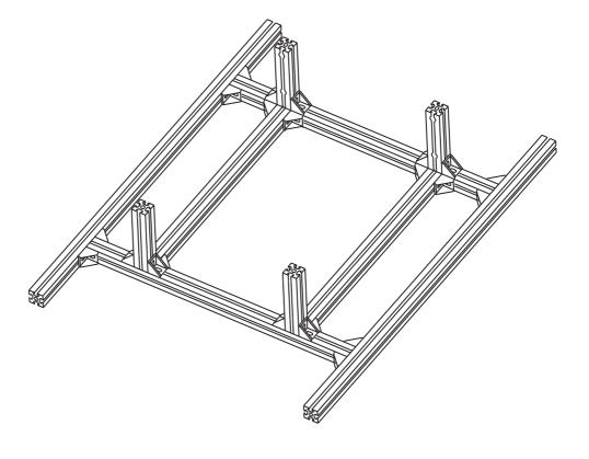
4. Now, Fix the assembly to the frame that we assembled in step (2) as per image. Here, we had completed assembly of chassis frame.
