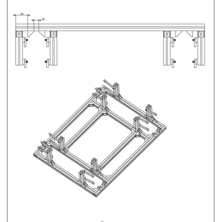
7. We will fix 98mm Metal Shock Absorber to the corner brackets mounted in last step. For this, we will use 10mm spacers, M4X20 Allen bolt & M4 Nyloc Nut with 8 qty of each. Mount all Shock Absorber with the help of the 10mm spacer. Make sure it was mounted with correct orientation. (Refer fig.)
