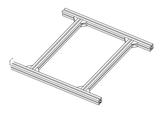
2. Now, fix 4 pieces of 100mm length 20X20 extrusion as shown in below fig. Also fix it separately on 380mm extrusion as shown in image, we will use it after some time. Make sure orientation of the extrusion while fixing the extrusion.
