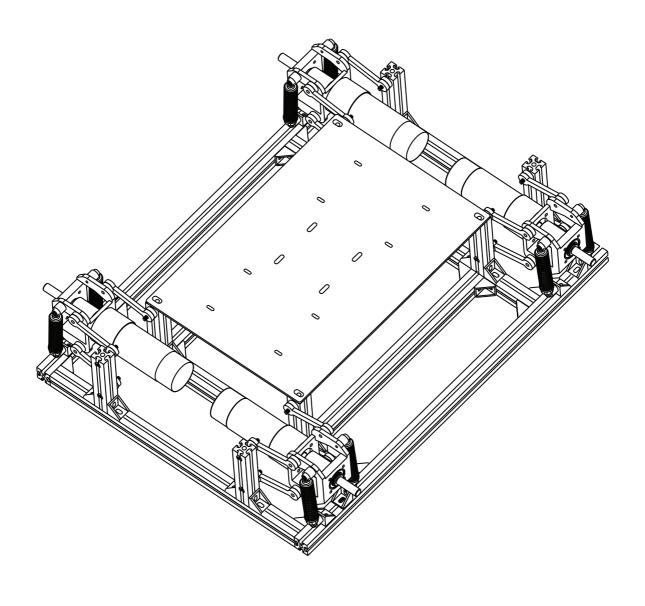
12. Now, Fix the 10mm Antislip Coupling to the 152mm Mecanum Wheel with the help of M5X65 Allen Bolt & M5 Nyloc Nut. Attach the Wheel Assembly to the Bearing Housing Shaft. Tight the M4 bolts on the flange side of the coupling. Tight it gradually. Apply the same procedure for rest of the Wheels.
