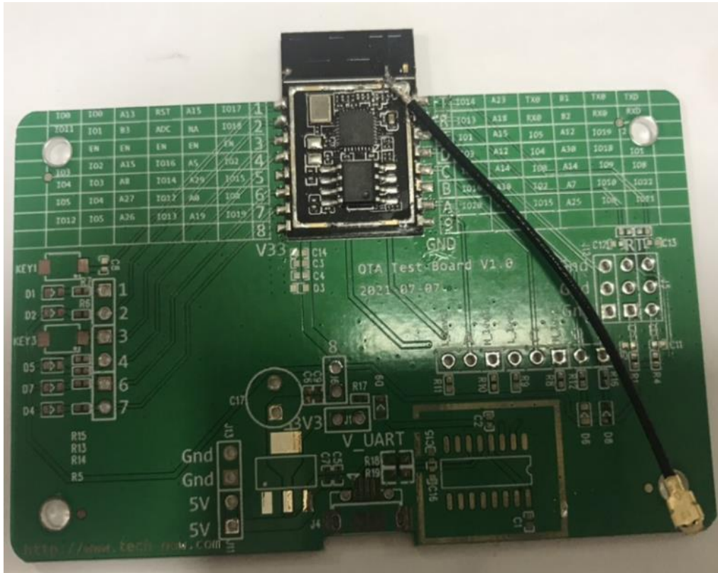
Figure 8 Schematic diagram of the antenna test prototype
