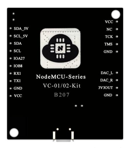
Figure 6 Development board pin diagram (bottom view)
