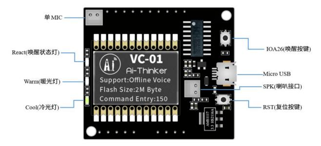
Figure 5 VC-01-Kit indicator light and button position
