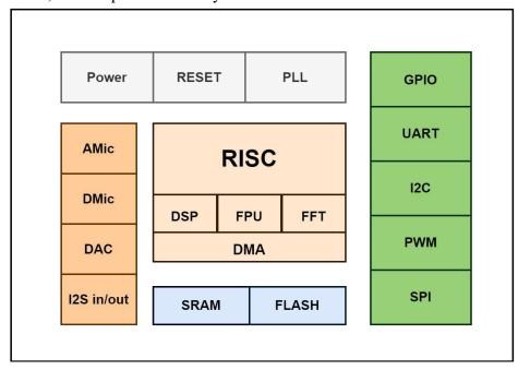
Figure 1 US516P6 chip architecture diagram
