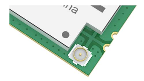
At the same time enable IPEX interface and stamp hole interface, IPEX interface and stamp hole interface can be arbitrarily selected
