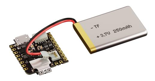
Example of a typical solution for remote machine vision including an Arduino® Nicla Vision and LiPo battery.
