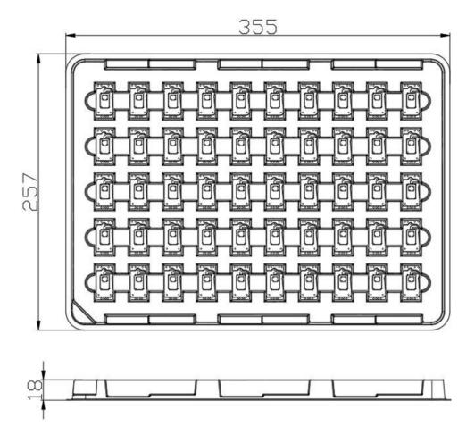
Figure 5. Size of plastic tray (unit: mm)
