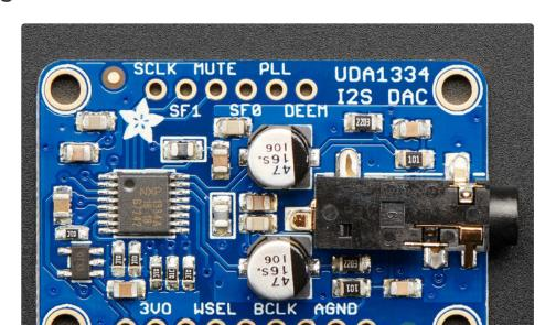
The UDA1334A is an **I2S** amplifier - it does not use analog inputs, it only has digital audio input support! Don't confuse I2S with I2C, I2S is a sound protocol whereas I2C is for small amounts of data.
