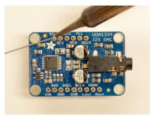
Solder each one of the pins into the board to make a secure connection
