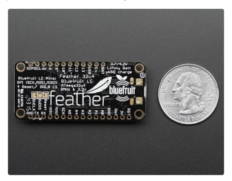
To make it easy to use for portable projects, we added a connector for any of our 3.7V Lithium polymer batteries and built in battery charging. You don't need a battery, it will run just fine straight from the micro USB connector. But, if you do have a battery, you can take it on the go, then plug in the USB to recharge. The Feather will automatically
