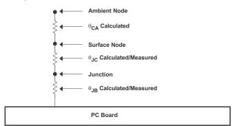
Figure 11-2. Thermal Resistance
