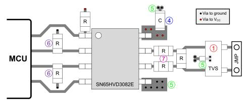
Figure 11-1. SNx5HVD308xE Layout Example
