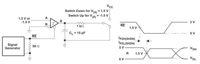
Figure 7-12. Receiver Enable From Shutdown Test Circuit and Waveforms
