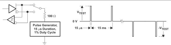
Figure 7-13. Test Circuit and Waveforms, Transient Overvoltage Test
