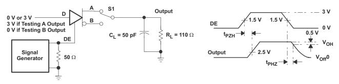
Figure 7-5. Driver Enable and Disable Test Circuit and Waveforms, High Output
