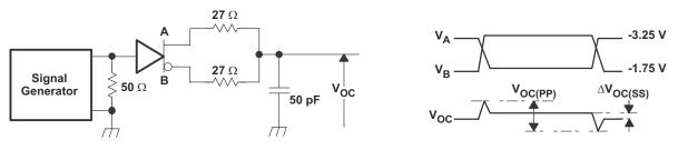
Figure 7-3. Driver V<sub>OC</sub> Test Circuit and Waveforms
