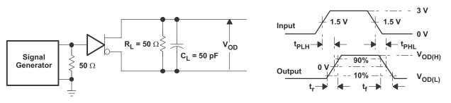
Figure 7-4. Driver Switching Test Circuit and Waveforms
