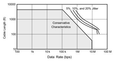
Figure 9-3. Cable Length vs Data Rate Characteristic
