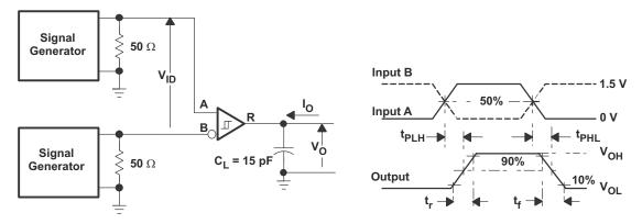
Figure 7-9. Receiver Switching Test Circuit and Waveforms
