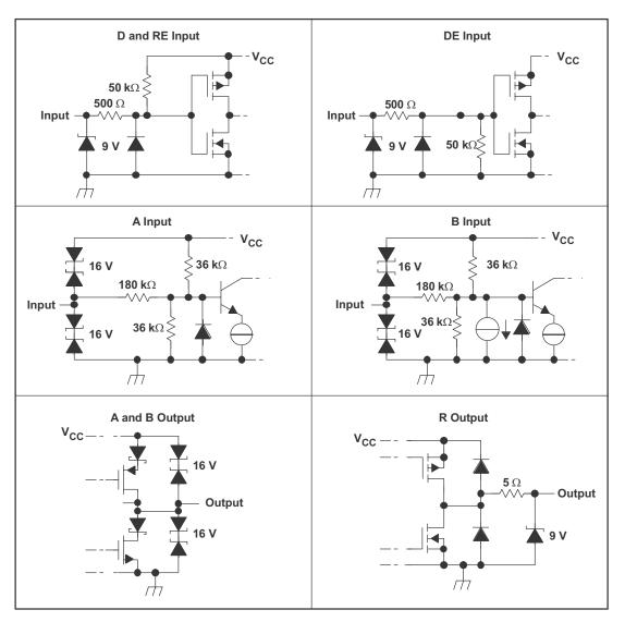
Figure 7-14. Equivalent Input and Output Schematic Diagrams
