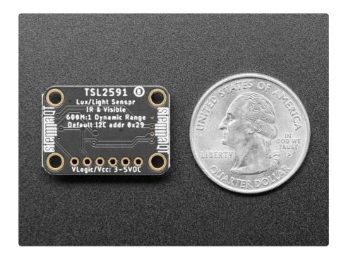
This sensor is much like the TSL2561 but with a wider range (and the interface code is different). This sensor has a massive 600,000,000:1 dynamic range! Unlike the TSL2561 you cannot change the I2C address either, so keep that in mind.
