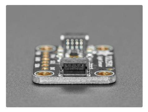
The built in ADC means you can use this with any microcontroller, even if it doesn't have analog inputs. The current draw is extremely low, so its great for low power data-logging systems. about 0.4mA when actively sensing, and less than 5 uA when in power-down mode.
