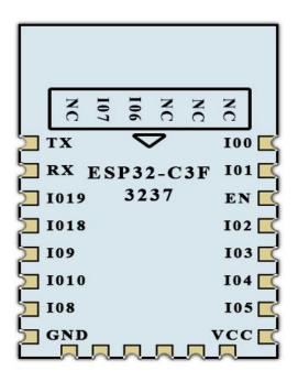
ESP32-C3F Diagram of Pin
