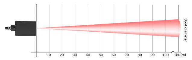
Figure 3 Detection angle schematic of TF03
