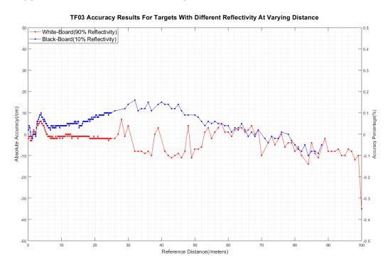
Figure 9 Error curves of TF03 at different distances and reflectivity
