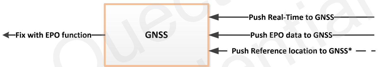
Figure 2: EPO™ Function Operation Flow
