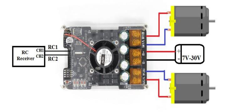
Sample Connection Diagram of RC receiver and motor with SmartElex 30D.
