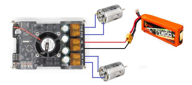
SmartElex 30D can be used with power supplies or batteries. Input power is connected to the center power terminals labeled B+ and B-. The input voltage range is 7V to 30V. The input current is dependent on the motors being used and the load placed upon them.
