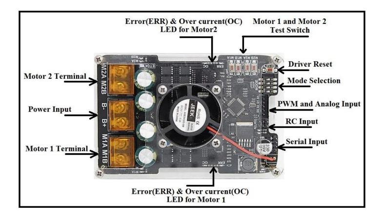
Power Input: Connect to a 7V-30V Battery or Power Supply.
