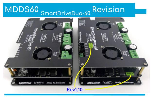
**Note:** MDDS60 is shipped in **Rev1.10 since January 2019**. There is a component changes on the circuit. The modification does not affect the performance or the interface.
