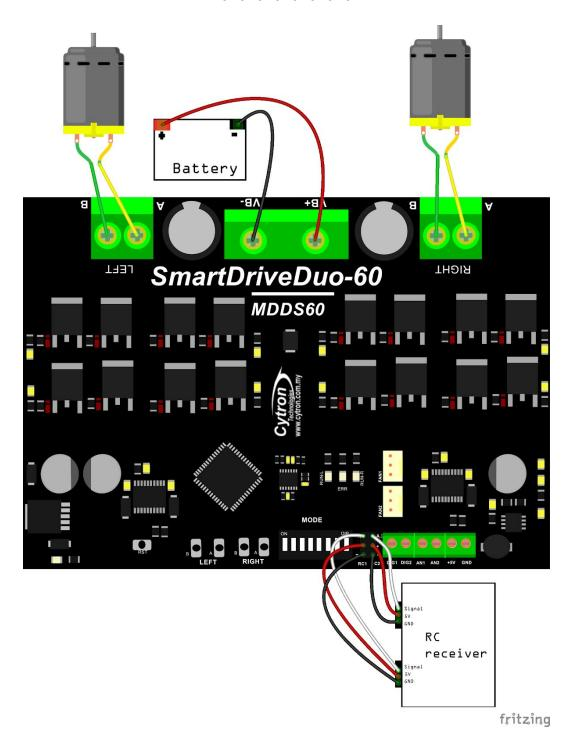
RC Mode with Microcontroller (Independent Both), DIP switch
