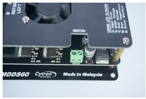
As shown in the picture above, there is terminal block for external power switch. Here are the steps on how to add external power switch.
